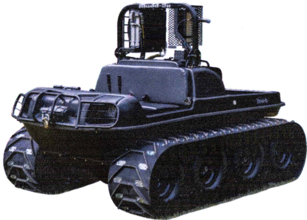
Fort Mac: Industrialized brute strength. Designed specifically for high demand applications by eliminating chain and bearing maintenance on the axles. Four individual hydraulic wheel motors directly drive the track system.
