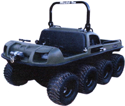
Vengeance: The answer to a cost-effective, nimble 8x8 amphibious ATV. Vengeance uses CVT clutches to power a twin planetary transmission for true all-wheel drive and smooth turning. Various gasoline EFI engines are available.
