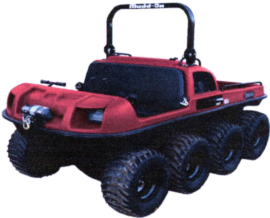
XL: A true workhorse. The Kubota engines directly drive a hydrostatic driveline for precision handling in extreme conditions and hill descends. Instant forward/reverse and counter rotation.
